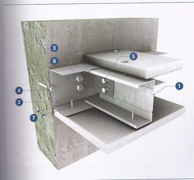
Ceiling perimeter framing at junction with masonry wall (applicable for ceiling span above 3000mm)
