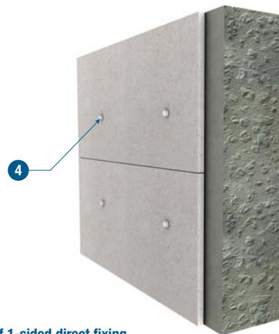
Details of 1-sided direct fixing
