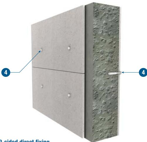
Details of 2-sided direct fixing
